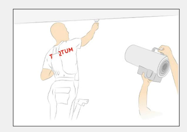
The suspended sheet is heated by heat cannon - heat causes the film to become soft and malleable
